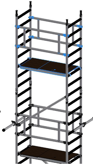
17) Fit a trapdoor platform to the 6th rung down from the top when installing on a FKS4/8. Then from a 3T position install 2 guardrail frames.
