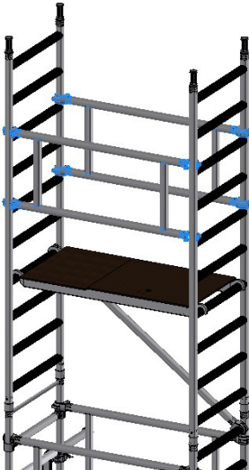
13) Sitting through the platform, fit 2 guardrail frames, one either side or 4 Horizontal braces 2 either side with hooks facing out.
