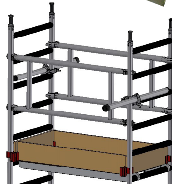
20) Then fit your toe-boards. This can either be a folding toe-board or the blank lengths with clips depending on which kit you choose.
