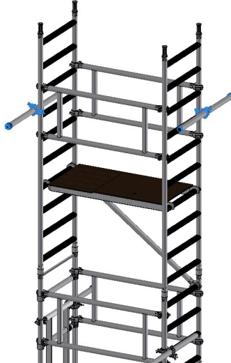
14) Fit 2 side props every 2m, one either end of the tower. If you cannot fit side props, stabilizers shall be fitted to all 4 corners of the tower. They shall be fitted to create the largest footprint possible.
