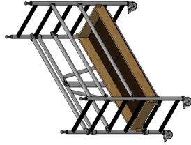
0.55m (Use guard locator above rung 3 and 5th rung)
