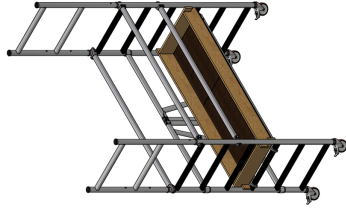
0.85m (Use guard locator above rung 4 and 6th rung)
