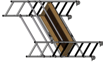
1.15m (Use guard locator above rung 5 and locator above rung 6)
