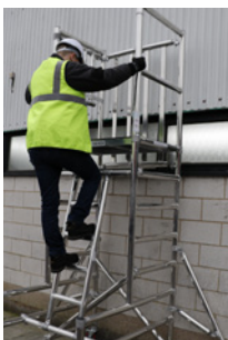
Access the platform using the step platform and ladder, keeping 3 points of contact with the unit at all times.
