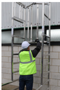
Open the unit on a firm and level base, lock the folding section.
